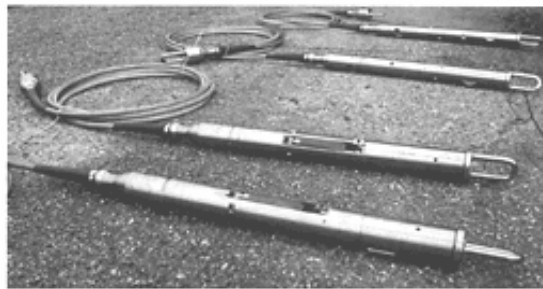
Figure 11: Satellites of the SST 500 tool (CGG)
